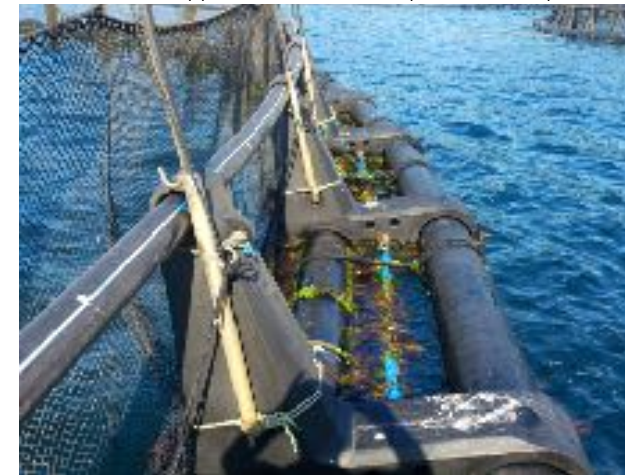
Toford's Anti-Flyer Stanchion without the bird net pole
