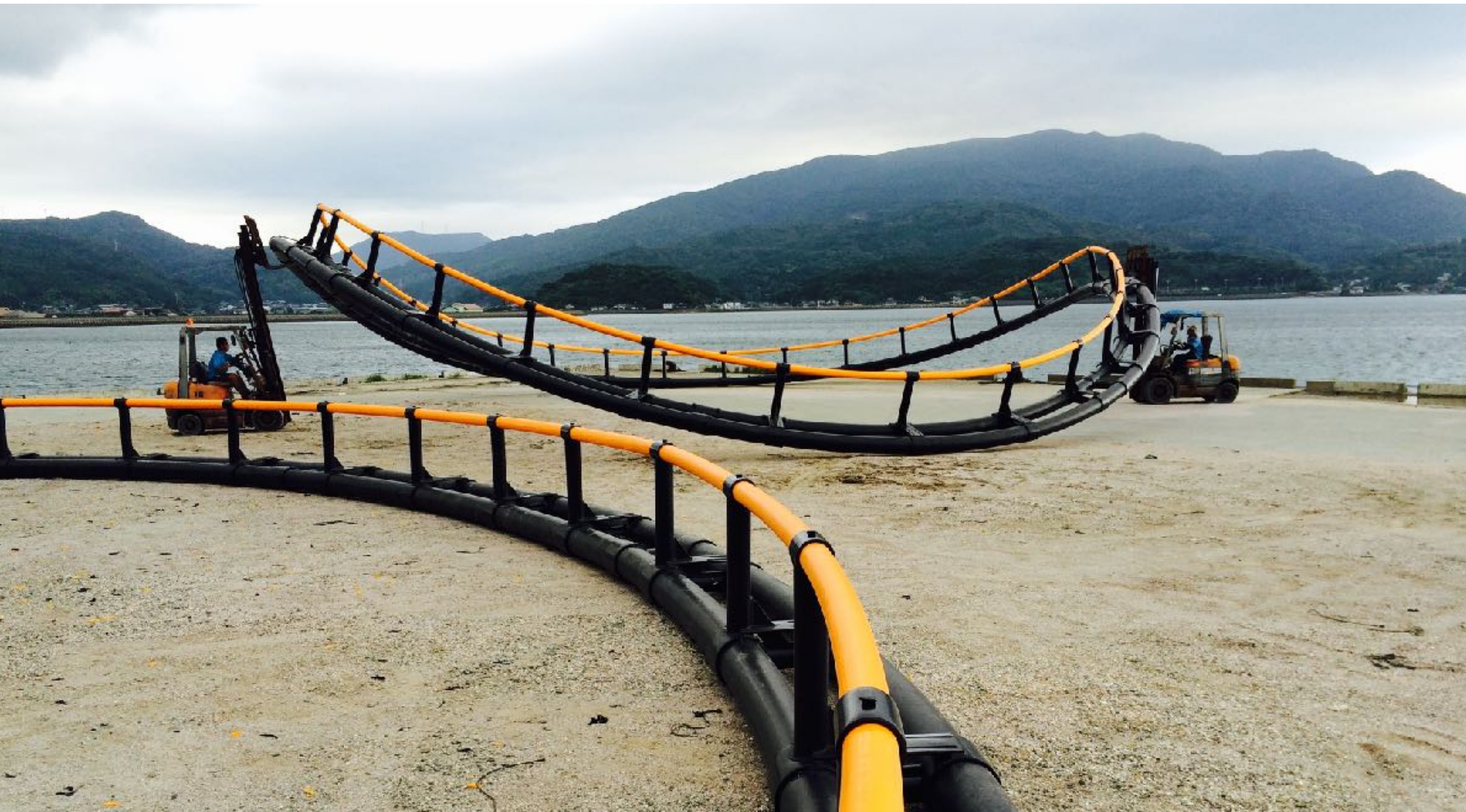
Standard 20m diameter cage with 250m stanchions - Amakusa, Kyushu, Japan
