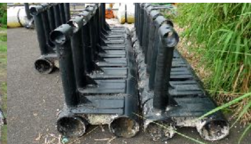
Cage damaged by cargo ship. Undamaged components are extracted to be reused.
